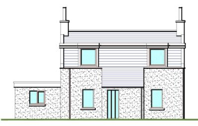
CONCRETE ROOF TILES - GREY UPVC WINDOWS & DOORS - GREY UPVC DOWNPIPES - BLACK WHITE RENDERED FINISH TO WALLS ETERNIT CLADDING TO PORCH - GREY
